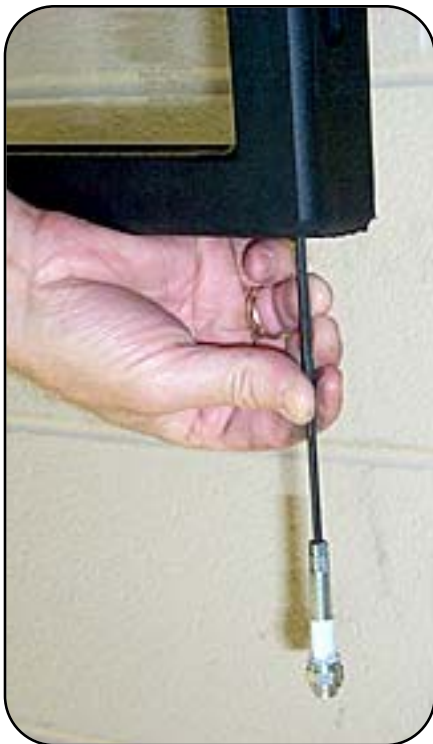
Figure 8. Replacing Door Hinge Spring Assembly
